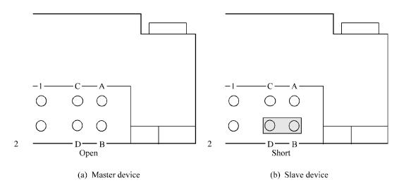
Figure 3.11 Jumper setting of master or slave device
